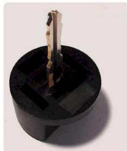
2. With care, use pliers to snap apart the plastic handle. Note most OEM keys contain a RF immobilizer chip in the center or on the side of the plastic handle. Use caution when taking apart, do not damage the RF immobilizer chip if it is required for immobilizer bypass installation method 2.
