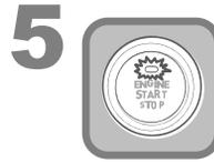
Button LED will flash Green / Amber alternately to indicate programming mode is active.
